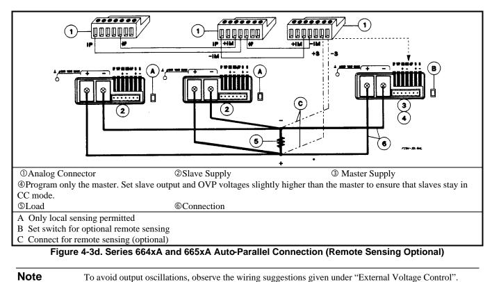
**Auto-Parallel Programming.** Program only the first ("master") supply in the series; the "slave" supplies automatically track the master's output. However, the voltage and OVP settings of the slave supplies must be set higher than the operating voltage of the master supply. This ensures that the slave supplies will operate in CC mode. Functions such as status, voltage readback, and current readback can still be read back individually for each supply.
